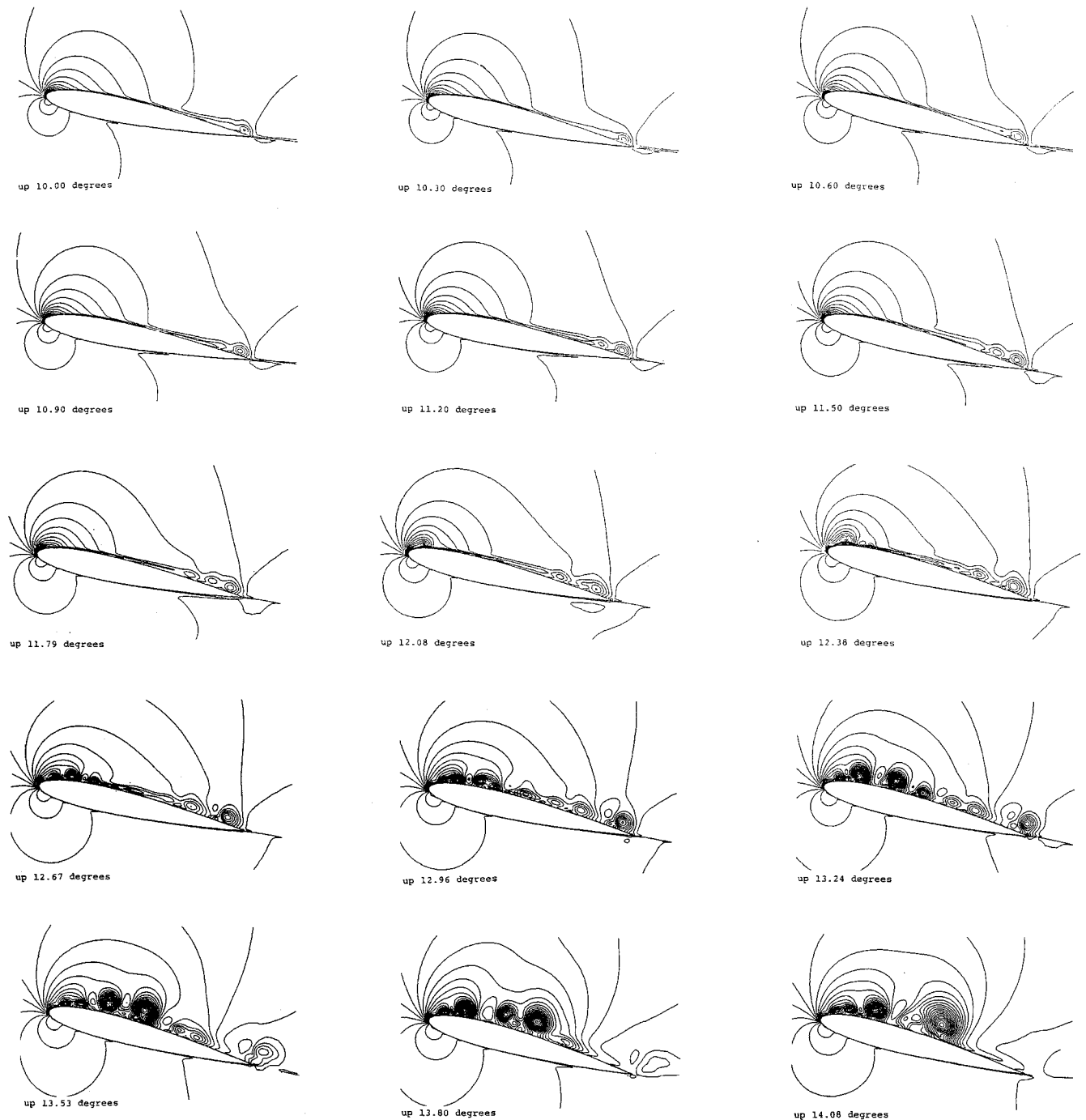
Fig. 5 Density contours at the beginning of separation at stall stage in the case of 321 \times 80 mesh.
